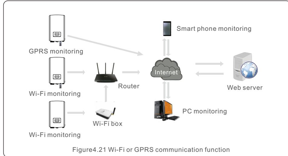
Figure 4.21 Wi-Fi or GPRS communication function
