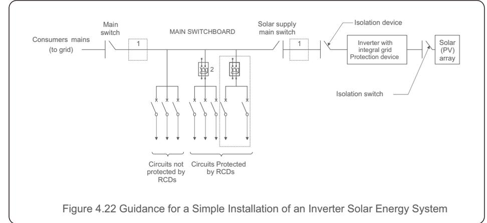
Figure 4.22 Guidance for a Simple Installation of an Inverter Solar Energy System
