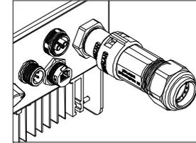
Figure 4.19 Connect the AC Connector to the Inverter
