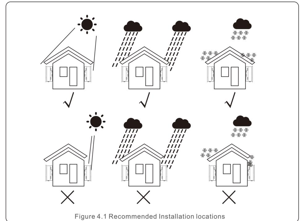
Figure 4.1 Recommended Installation locations
