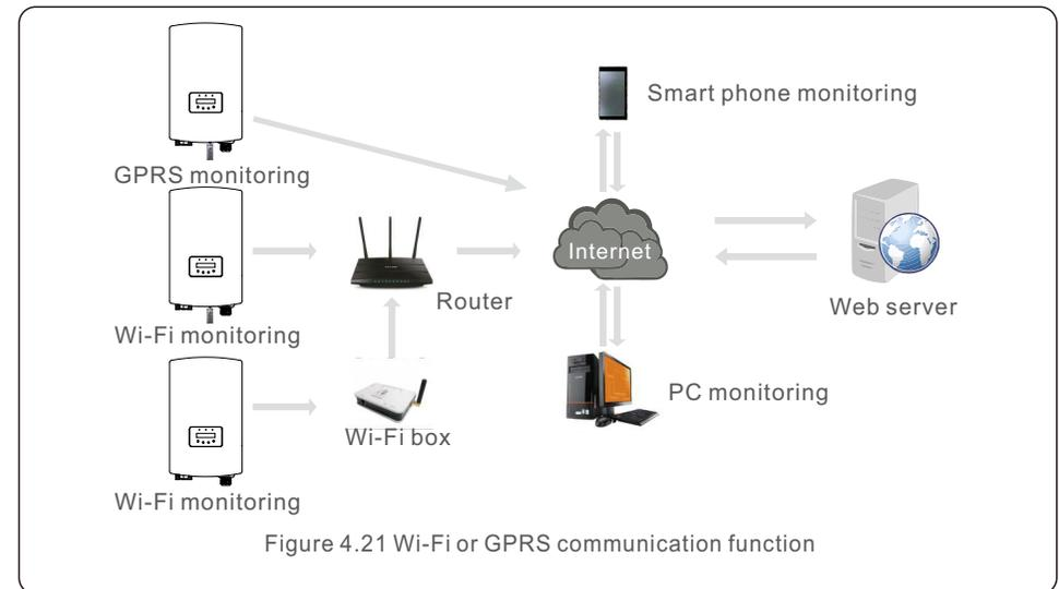
Figure 4.21 Wi-Fi or GPRS communication function
