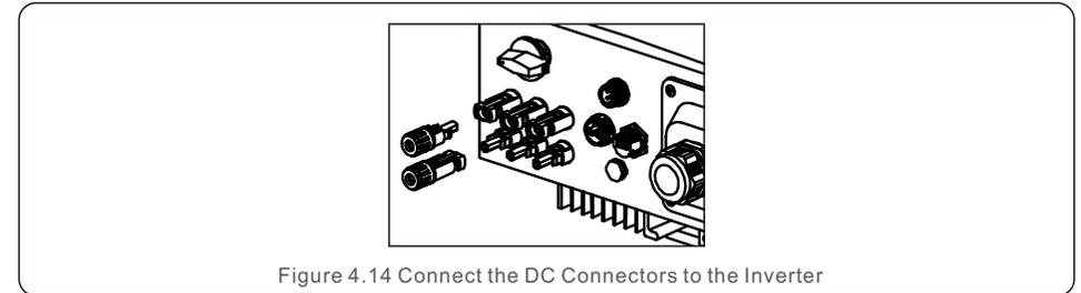
Figure 4.14 Connect the DC Connectors to the Inverter
