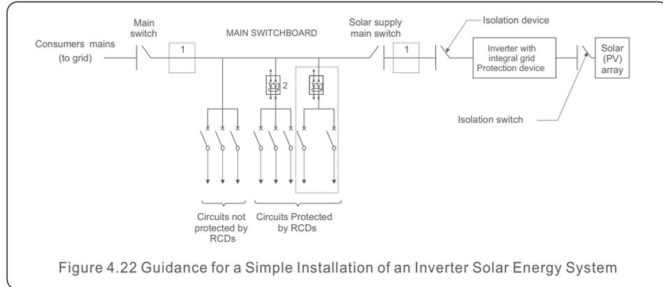
Figure 4.22 Guidance for a Simple Installation of an Inverter Solar Energy System
