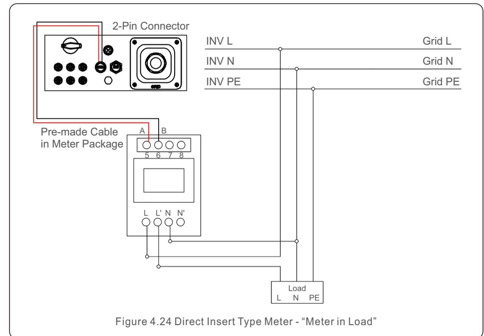
Figure 4.24 Direct Insert Type Meter - "Meter in Load"
