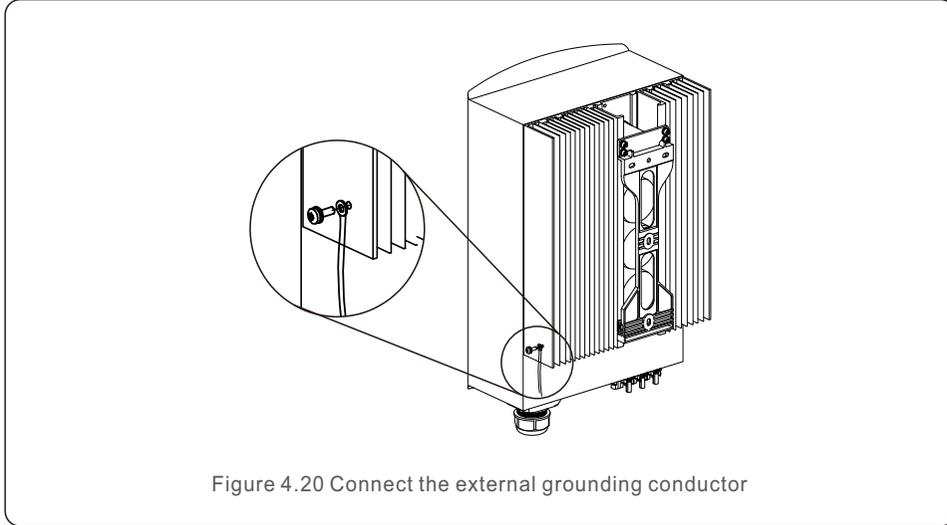
Figure 4.20 Connect the external grounding conductor
