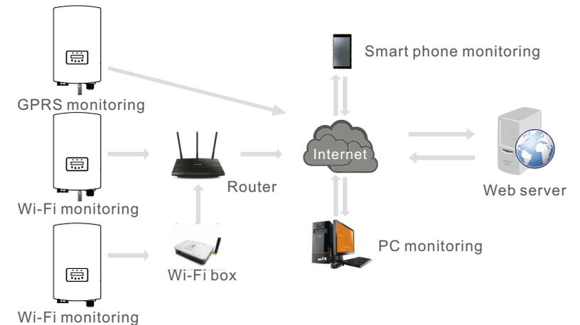
Figure 4.21 Wi-Fi or GPRS communication function
