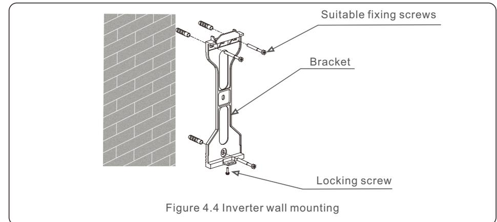
2. Make sure the bracket is horizontal and the mounting holes (in Figure 4.4 and Figure 4.5) are marked correctly. Drill the holes into the wall or pillar at your marks.
