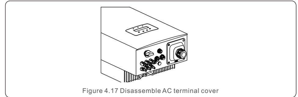
Figure 4.17 Disassemble AC terminal cover
