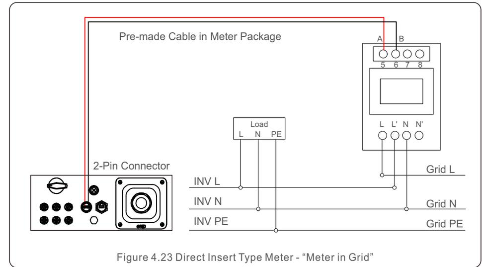
Figure 4.23 Direct Insert Type Meter - "Meter in Grid"
