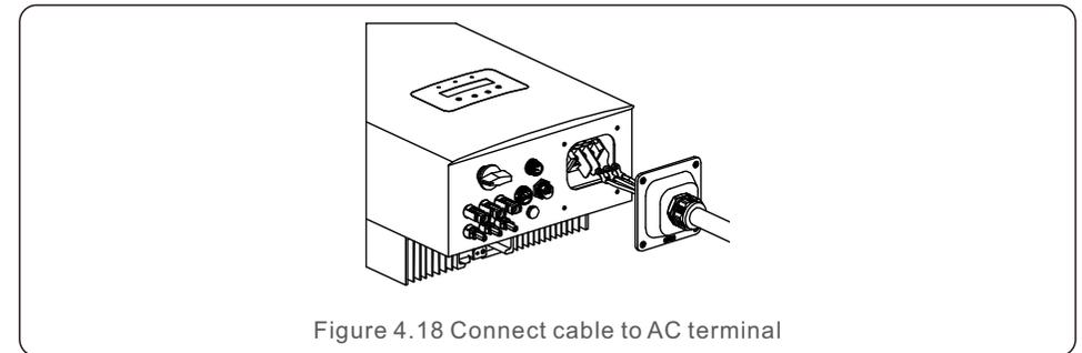
Figure 4.18 Connect cable to AC terminal
