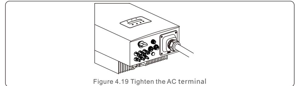
Figure 4.19 Tighten the AC terminal
