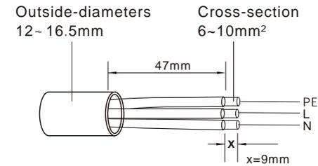
▲ Figure 4.15 Stripped AC Wires
