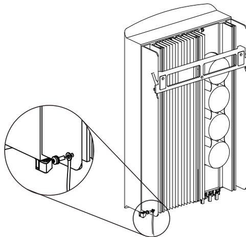
▲ Figure 4.19 Connect the external grounding conductor
