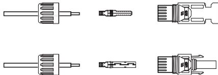
▲ Figure 4.8 Disassemble the Connector Cap nut
