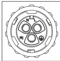
▲ Figure 4.13 AC Grid Terminal Connector Inside
