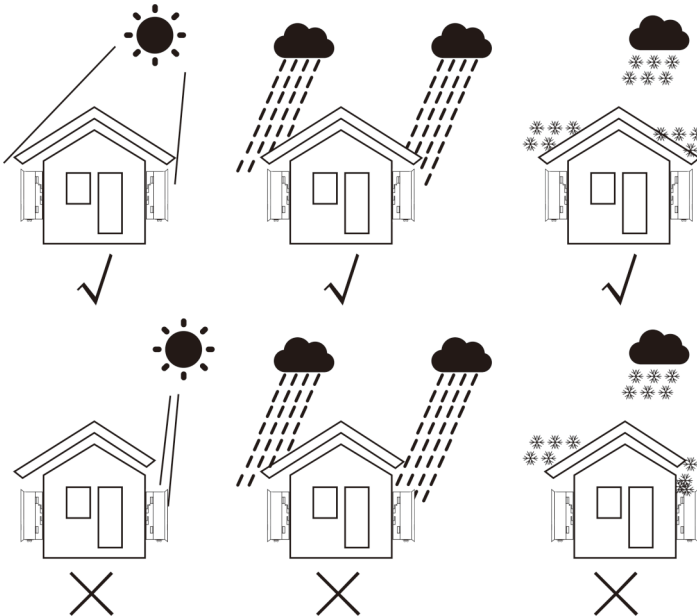
Figure 4.1 Recommended installation position
