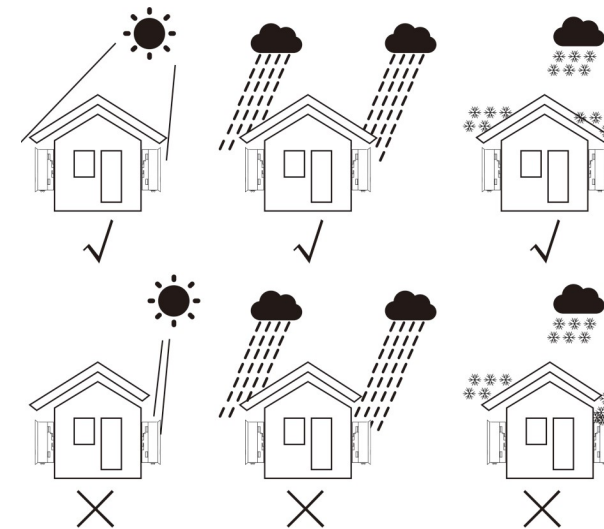
Figure 4.1 Recommended Installation locations
