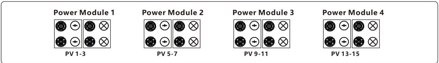
If four power modules are indeed required to connect the solar panels unevenly, for a power module which is connected to no more than three strings, it is necessary to ensure that the power of each PV string connected under this power module does not exceed 7.6kW to achieve better power generation performance. In the case that the power difference between each PV string is less than 10%, the 3 common cases are showing below.
