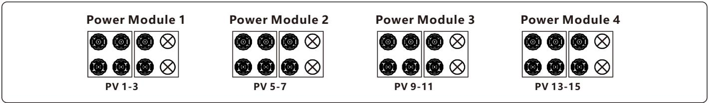
If four power modules are indeed required to connect the solar panels unevenly, for a power module which is connected to no more than three strings, it is necessary to ensure that the power of each PV string connected under this power module does not exceed 7.6kW to achieve better power generation performance. In the case that the power difference between each PV string is less than 10%, the 3 common cases are showing below.
