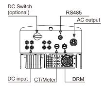
If no PV string connects to the DC input terminals, please install the watertight cap onto the empty DC input terminals to guarantee the inverter ingress protection rating.
