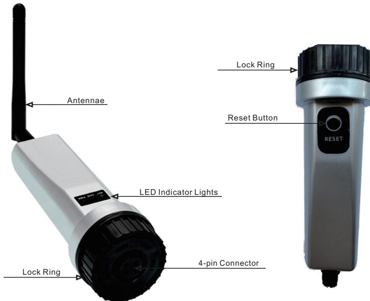
Figure 1.1 Logger Parts
