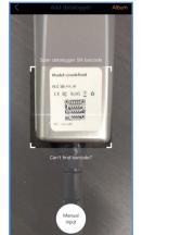
Note: Scan the datalogger SN, NOT the inverter SN.
