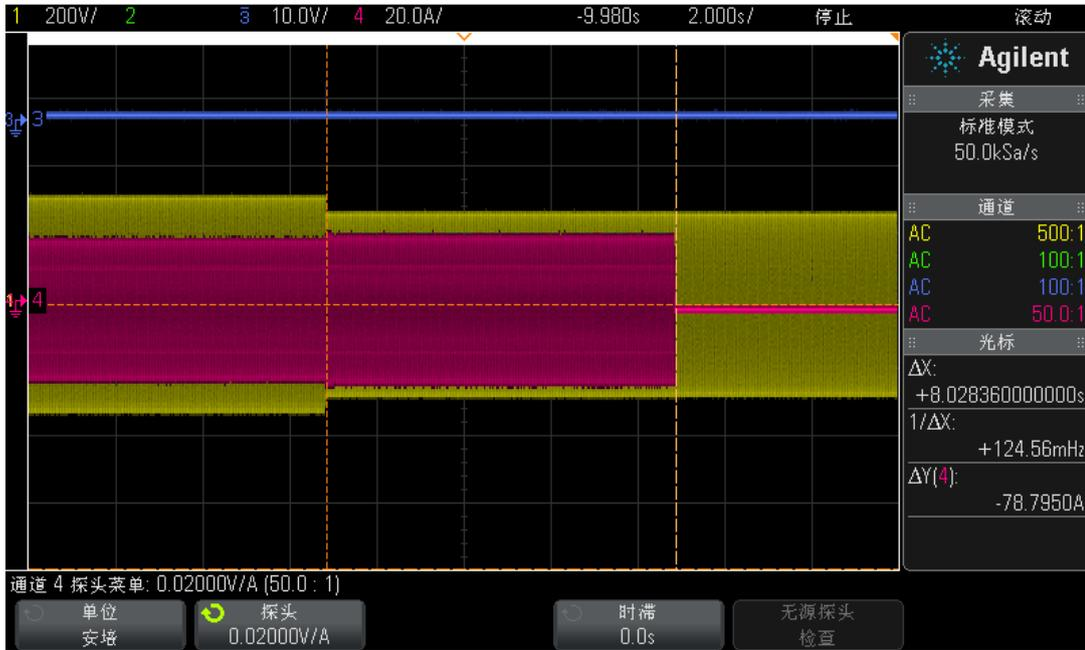
Disconnection Time - Over Voltage First Level
