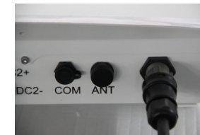
▲ Figure 4.14 Connect the Terminal Connector to GCI-4.6K-W
