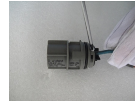
▲ Figure 4.12 Connect Wires to the Grid Terminal
