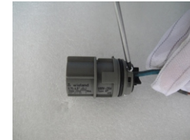
▲ Figure 4.12 Connect Wires to the Grid Terminal
