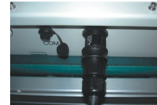
▲ Figure 4.14 Connect the Terminal Connector to GCI-3K-DB
