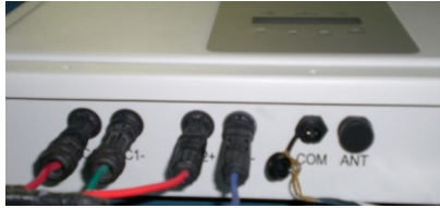
▲ Figure 4.9 Connect the DC Connectors to the Inverter
