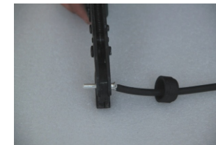
▲ Figure 4.7 Attach the Pin Top to the wire
