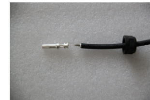
▲ Figure 4.6 Insert the Wire into the Connector Cap
