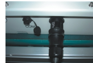
▲ Figure 4.14 Connect the Terminal Connector to GCI-1.5K
