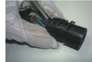
▲ Figure 4.12 Connect Wires to the Grid Terminal
