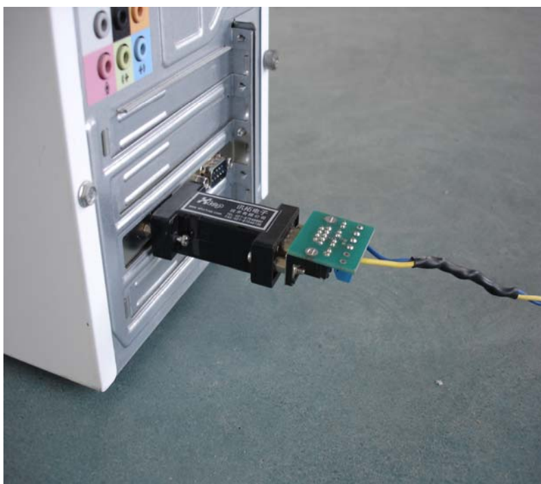
Picture 6. RS485/RS232 Converter connected with PC
