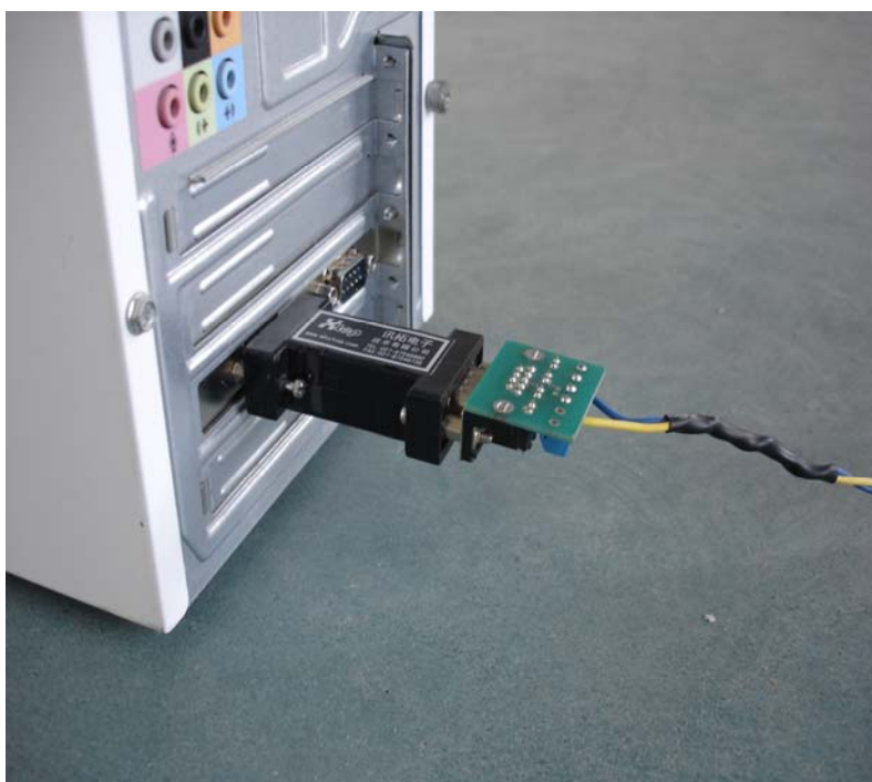
Picture 6. RS485/RS232 Converter connected with PC
