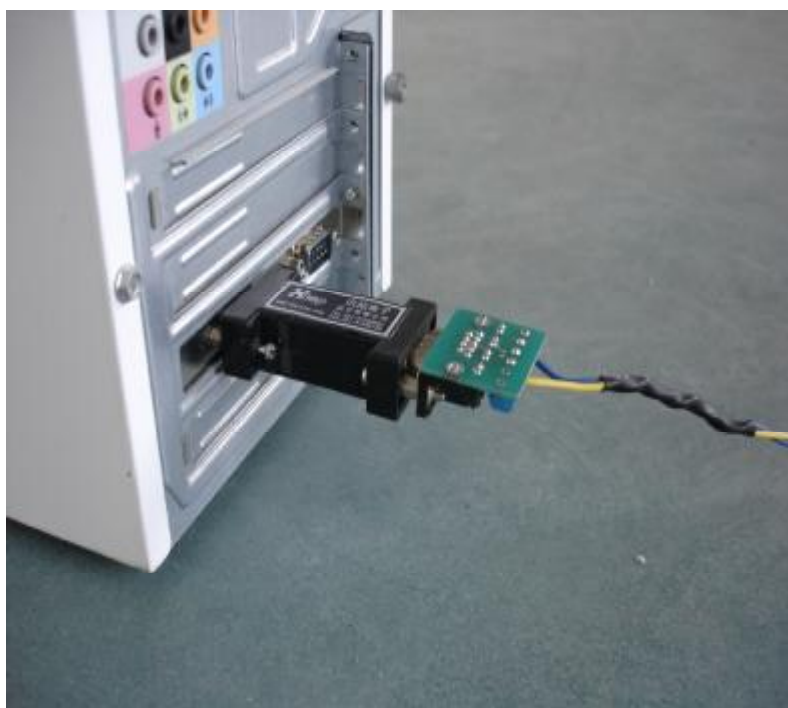
Picture 6. RS485/RS232 Converter connected with PC
