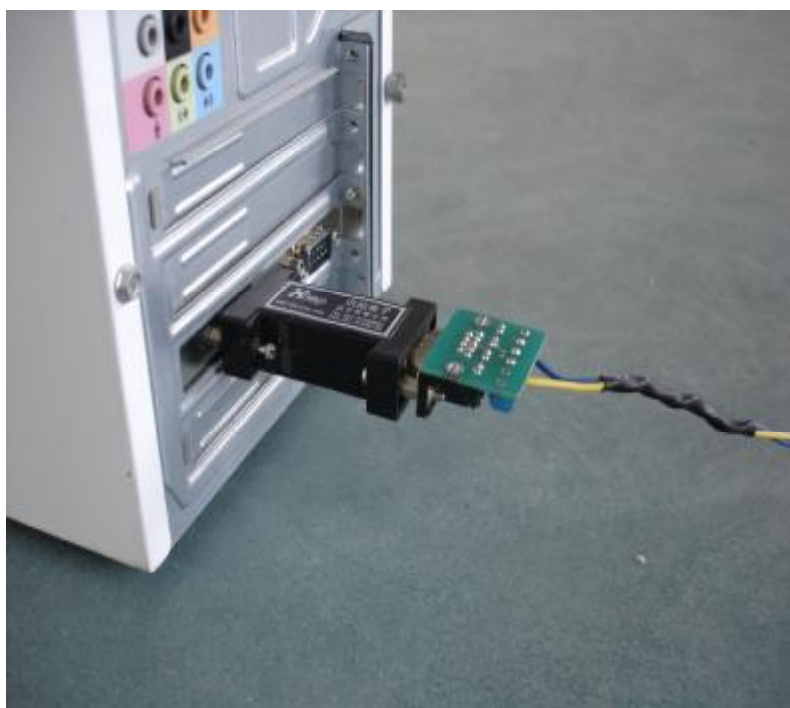
Picture 6. RS485/RS232 Converter connected with PC
